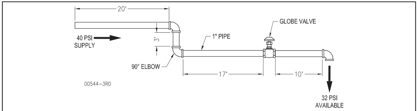
Total of above = 20 + 2.2 + 3 + 2.2 + 17 + 23 + 10 + 2.2 = 79.6 feet. Since each 10 feet is equivalent to 1 psi pressure loss, 79.6 feet is equivalent to approximately 32 psi from an original Boiler supply of 40 psi.
