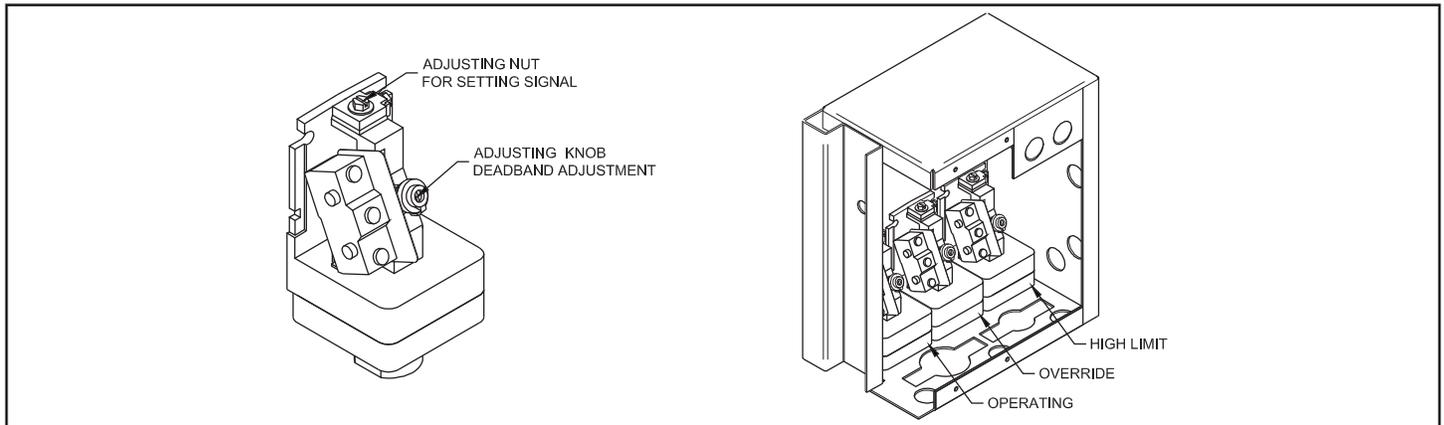
1. Turn the adjusting knob clockwise to the deadband to maximum.
