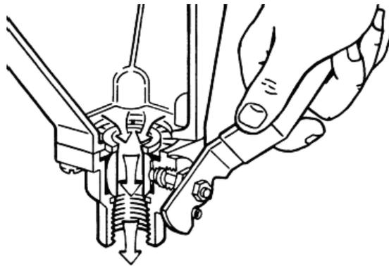
The Boiler Water Level Control installed on your boiler requires periodic maintenance. As boiler water circulates into the float chamber, sand, scale and other sediment may be deposited in the float chamber. While the chamber has been designed with a large accumulation bowl, it is necessary to flush the sediment from the chamber by blowing down the control so that the accumulation of sediment does not interfere with the movement of the float in the control.
